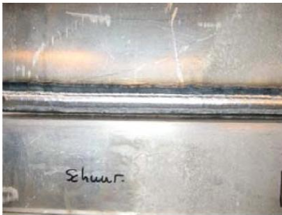
Seam smoothed using a stainless steel brush
