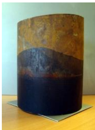
Rusty carbon steel pipe immersed in Rust Converter Super. The inert result was obtained in 2 hours (ambient temperature of 20°C and atmospheric humidity of 85%)
